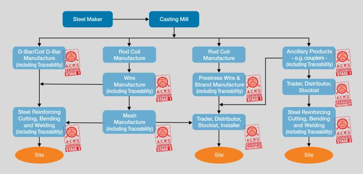
For reinforcing steels, ACRS certifies BOTH the steel mill that manufactures the steel AND the steel reinforcement processor and mesh supplier. Verification of the outputs of both these supply streams is essential for any steel reinforcing materials claiming to conform with the Standards.
